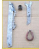
Fig 3: chain whip, cassette removal tool, 1" thin wrench, spoke wrench.
