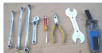
Fig 7. l to r: (a) 6-8 mm box end wrench, (b) 7-9 mm box end, (c) 10-11 mm box end, (d) 4 1/2" adjustable wrench, (e) 4" flat-bladed screwdriver, (f) 5" needlenose pliers, (g) 15-16 mm cone wrench, (h) 1.5 mm, 2mm, 2.5mm, and 3 mm allen wrenches.
